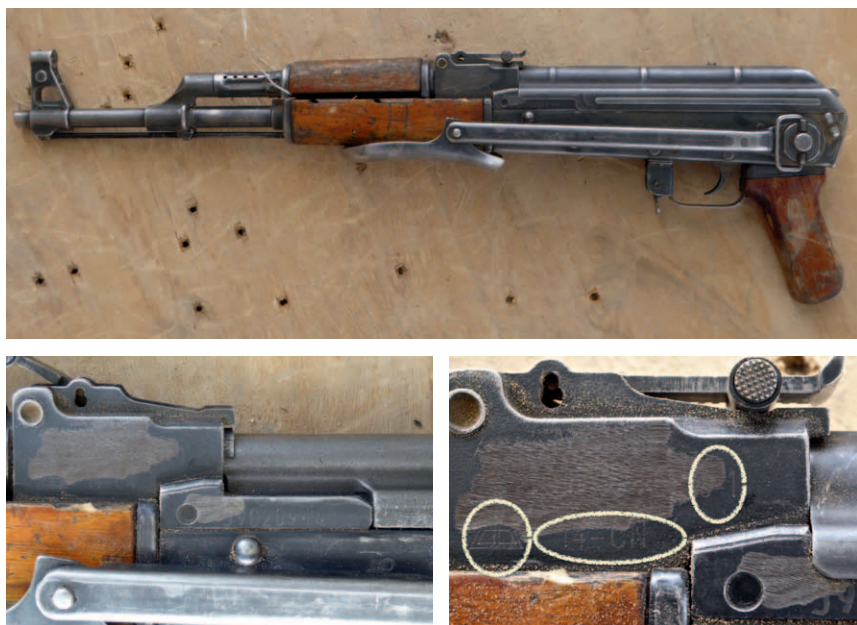
Photos 22–24 Close-up of the markings on the rear-sight block and on the receiver of the Type 56-1 rifle with the serial number 59020947, documented on 2 March 2017, in Dirkou, Niger. The bottom of the inscription '56-1', of Factory 26 logo (26 inside a triangle), and of the inscription '14-CN' remain visible despite abrasion marks.
